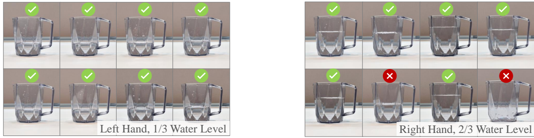
Figure 10: Visualization of the resulting water levels across 8 trails in Pour Water-L-1/3 and Pour Water-R-2/3 . Left: The water level completed by RDT in each trial is extremely close to the ground-truth 1/3 standard. Right: RDT made one mistake in pouring (empty cup) and one mistake in water level, but the other trials were in roughly good agreement with 2/3.
